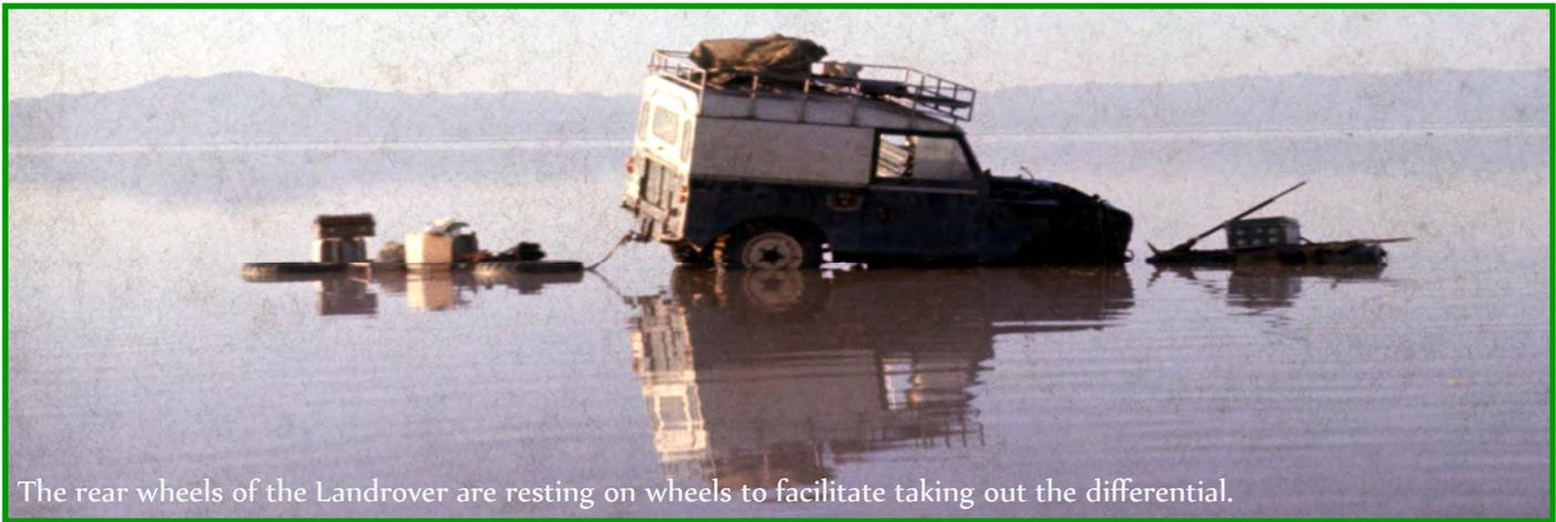
The rear wheels of the Landrover are resting on wheels to facilitate taking out the differential.
